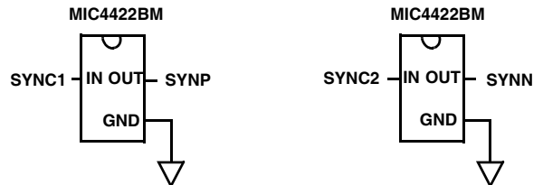
FIGURE 22B. NON-INVERTING DRIVERS
